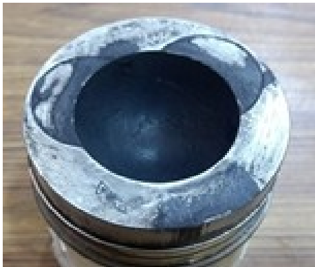
Fig. 1: Conventional Engine Piston.
